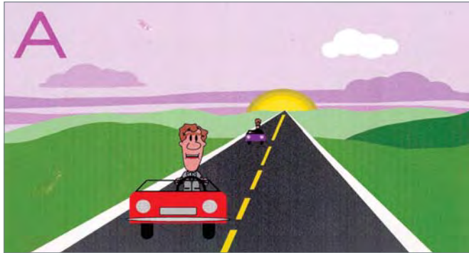
A Free Flow A general level of comfort and convenience provided to the motorist is excellent.
