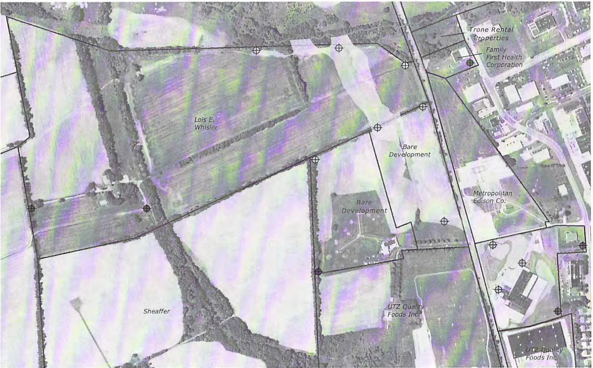
Figure 2-1 Proposed Groundwater Monitoring Wells Miller Chemical & Fertilizer, LLC, Hanover, PA
