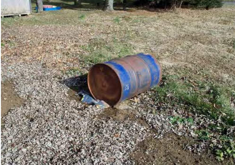
21. VIEW OF 55-GALLON DRUM WITH OBSERVED BULGING
