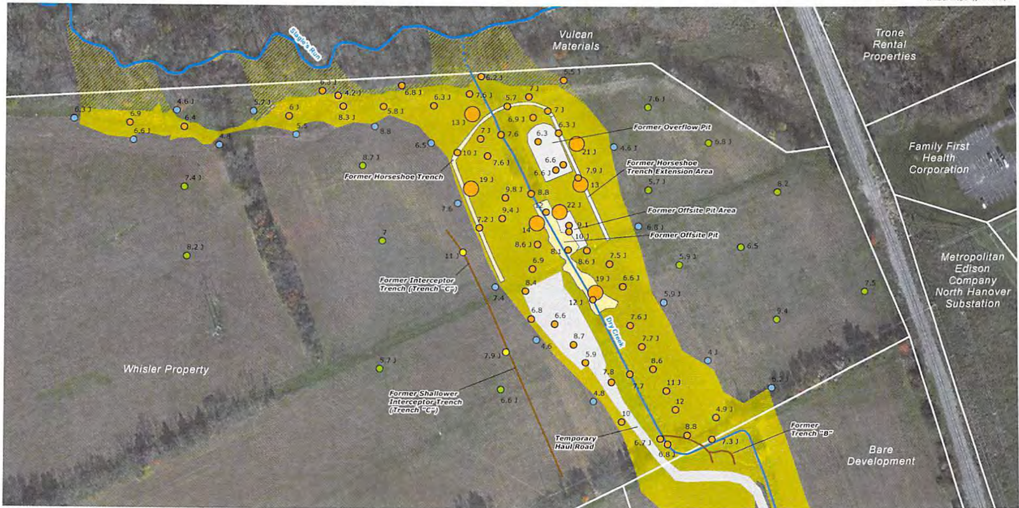
Figure 5-1 Summary of Maximum Measured Arsenic Concentrations in Soil Whisler Property, Hanover, PA
